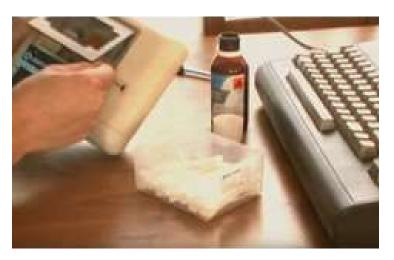
Don't forget to clean the erasehead too, although you don't need it for reading back tapes it is very important for writing. When cleaning of both heads is done, make sure to let it dry for at least 15 minutes before using it, you don't want your tapes to get wet OR to stick to your wet tapehead while recording/playing.
