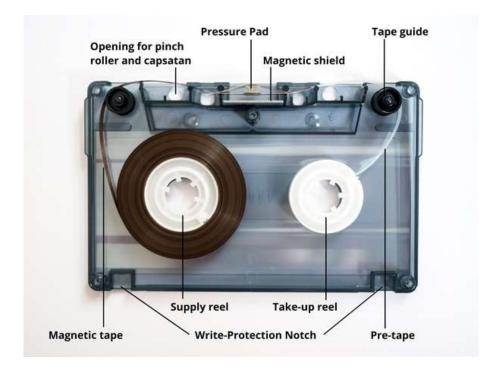
Tapes have a write protection notch on their edge. If it is open (removed) a recording cannot be made. If this notch is open, place a piece of adhesive tape to allow for a recording to be made. It may be a good idea, to remove the adhesive tape or (if still present) to break out the write-protect notch of the tape. Because accidentally erasing the content by another recording will be prevented.
